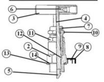
1"600lb Serrated Face Flanged Double Block & Bleed Valve [Needle/ Needle Configuration] with PTFE/17-4PH Trim. 1/2"NPT [F]Outlet/1/4"NPT [F] Vent in 316ss
